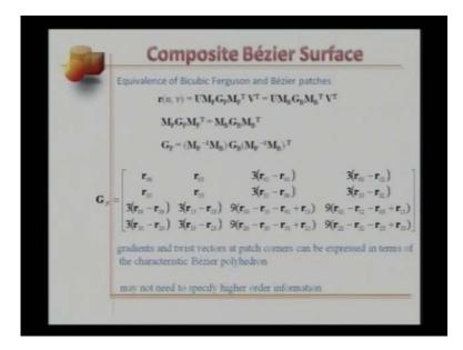
So, in terms of the design points that we have seen pertaining to G sub B, we can get the geometric matrix for the corresponding bicubic ferguson's patch. First row, is r 0 0 r 0 3,
