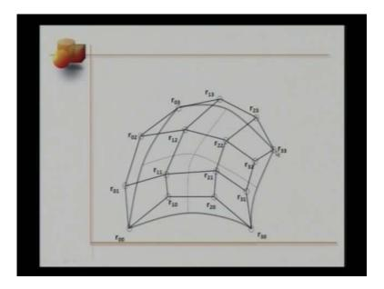
Let us revisit bicubic bezier patch with control points horizon points, r 0 0, r 1 0, r 2 0, r 3 0, r 0 1, r 1 1, r 2 1, r 3 1, r 0 2, r 1 2, r 2 2, r 3 2, and r 0 3, r 1 3, r 2 3, and r 3 3.
