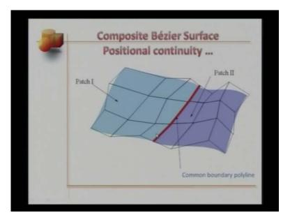
Here is the figure this is the control net for the first i cubic dispatch and this here is the control net for the second beziers patch; patch 1, patch 2. All the condition that we have seen in this slide says that the boundary polygon between these two nets should be the same, this here is a poly line.
