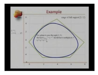
Now, if I would want to half my B spline curve pass through this design point 0 0, which is 3 plus 4 the fifth design point here. The knot t 4 plus four minus 1, which is t 7 is equal to 7, should have multiplicity 3. That means the knot values t 5, t 6 and t 7 they should same as 7. So my fifth data point or (()) point here and I would want my B spline curve to pass through b 4. That could mean I have to make N 4 8 equal to 1. I will have to do that by raising knot multiplicity.
