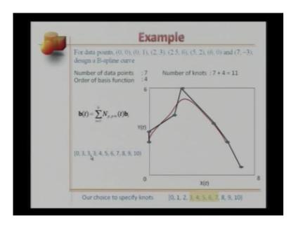
The B spline in red, now passes through the first control point all the design. Let us experiment further. Now, if we replace these knots t 8 and t 9, so that t 7 becomes a multiple knot of multiplicity 3, what happens then?
