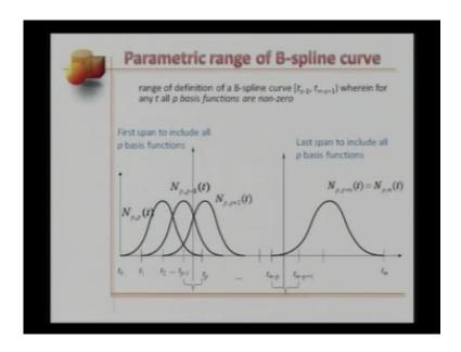
So, the range of the definition of a B spline segment will be given by until t m minus p plus 1 wherein for any t for any value of t all p basis functions are non zero. That means for values of t in between t 2 t m minus p plus 1 over this interval will be able to achieve full support of B spline basis functions. This would be the parametric range of B spline curve.
