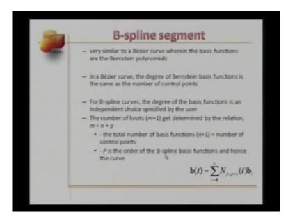
Now, a B spline segment is very similar to a Bezier curve or a segment wherein the basis functions are the Bernstein polynomials, I mention this before. This is the definition of a B spline curve or a segment. In a Bezier curve the degree of the Bernstein basis functions this is the same as the number of control points here. However, the degree or the order of the B spline basis function p is independent of the number of control points. In the sense p is not dependent on n.
