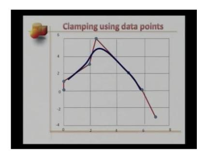
To clamp of B spline curve at the two end points we are working with this example throughout.
