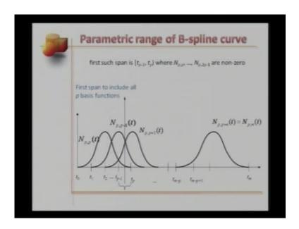
The first such span would be t p minus 1 t p, which is this 1 where N p p N p p plus 1 up till N p 2 p minus 1 are non zero. These are p B spline basis functions, which are non zero over this interval here. So, this would be the span to include all p basis functions.
