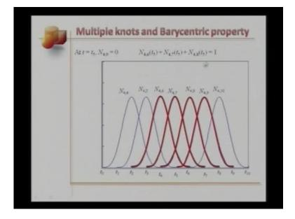
Let us see what we have with multiple knots Barycentric property. Let us say we have a set of knots going from t 0 until t 10, all simple knots. Correspondingly we have 1, 2, 3, 4, 5, 6, and 7 order 4 B spline basis functions. How would you name for sample this one? This would be N 4 4. Let us concentrate on these red shape functions for now. The B spline basis functions are named N 4 4, N 4 5, N 4 6, N 4 7 until N 4 10, you would know now how to do so.
