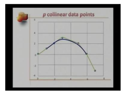
This one would be the new B spline curve. You would realize that a part of it forms a straight segment. This is because the convex hull defined by these four points de generates into a straight line.
