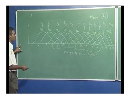
While you were busy sketching your B spline basis functions, I was sketching mine. So, this is the knots span t 0 up till t 15 uniform knots span with all simple knots at this time. This says the range of a support from 3 to 12 and these are my individual B spline basis functions N 4 4, N 4 5, N 4 6, N 4 7, N 4 8, N 4 9, N 4 10, N 4 11, N 4 12, N 4 13, N 4 14 and N 4 15. Now, remember an element in the summation when we define our B spline curve N p p plus i times b i.
