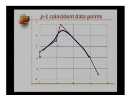
Now, the second case where p minus 1 data points or design points are co incident, that is there are the same. Let us look at the same example here this was the original B spline curve i move this point to coincide with this design point. Here this one again to coincide with these design points; so remember here this is an order 4 B spline curve p is 4 for as p minus 1 is 3. So, we have three design points which are coincidental what happens in this case.
