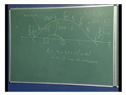
Let us try to construct an order 4 basis spline function, let me start with t 0, t 1, t 2, t 3, t 4 I would need 4 knot spans, this is the parameter axis t to the right and to the left. My B-spline basis function will start from t 0 and end at t 4, again I will have to be careful with
