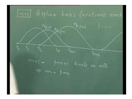
So, we have say n plus 1 B-spline basis functions each of order p, let us try to sketch them, we start with the knot t 0, the first one we sketch will be nomenclated as N p p. So, this knot here will be t p, the second one will start from t 1 will end at t p plus 1, this will be nomenclated as N p p plus 1. Likewise the third one, starts from t 2 ends at t p plus 2 and has the name N p p plus 2, I can keep doing this.
