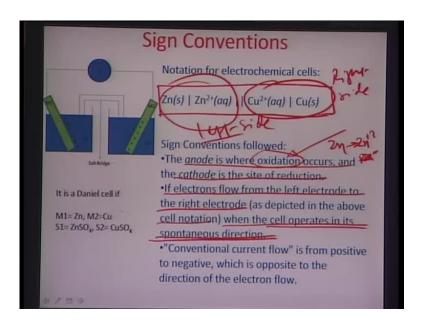
This is also a known as an electro chemical cell and in fact this is also called as a Daniel cell. So, what I would like to illustrate here is that there is a sign convention which is used for writing such half cells. The convention which is followed here is essentially, the
