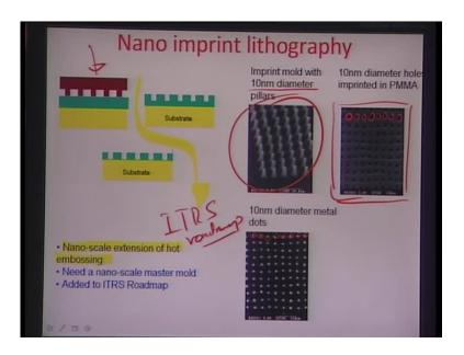
Another very important process which comes almost immediately from compression molding is Nano imprint lithography. I would like to illustrate that this process has also been made or be included in the ITRS road map especially, for the end of road devices.
