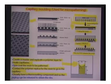
We are going ahead on this spree and try to finish the soft lithographic processes today, after which will do a little bit of introductory electro chemistry. The next process along the line is capillary molding; once again one of the important process especially for display technologies sometimes.
