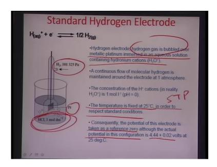
So, reference electrodes in this application has been universally accepted to be the standard hydrogen electrode which is essentially something like this, where there is a
