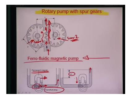
Now, there are other forms of pumping systems, one of them being rotary pumps with spur gears, as you can see here, in this illustration. Here, you see, there are two gears as you can see here; this is gear one, gear two. They are moving in a direction; this moves in anticlockwise, this is actually driven in the clockwise sense, as a result of which, the material which is inside this micro channel, gets pushed forward and flows in this direction.
