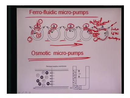
The third kind of pump is really very interesting, it is the ferrofluidic micro pumps. You have to really consider in detail the various stages from 1 to 5 of this particular pump and how it behaves. You have instead of one ferrofluidic plug, two plugs, essentially this particular illustration is one plug and this here as you see is the second plug.
