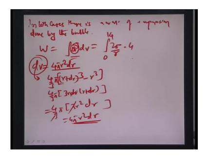
Let us say that in both cases there is a work of expansion which is done by the bubble and this work is essentially integral Pdv also this varies between 0 and 14 microns of course, and you have delta P here, the pressure differences is about 2 sigma by r times of the elemental volume as I had done way back before in case of spherical symmetry is given by 4 pi r square dr.
