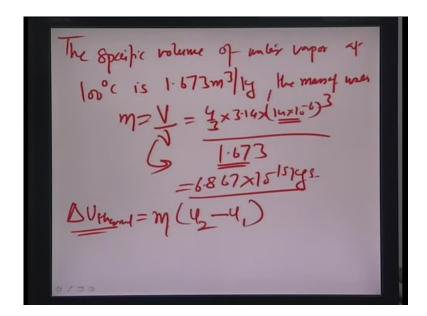
Let us try to look at that figure here and see what the mass would effectively be. In this case the mass comes to be about 6.867 into 10 to the power minus 15 kgs. Essentially, if you ignore the heat losses from the system, we assume that the system is hermitically sealed again. We can find out the thermal energy equivalent required for formulating this amount of water vapor mass 6.867 into 10 to the power minus 15 kgs of water vapor mass.
