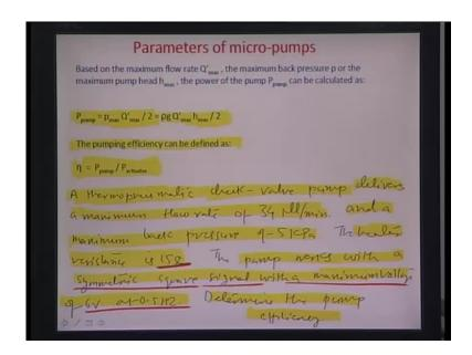
The electric power input here which causes the actuator power is half V square by R; V is 6 volts half because the half cycle is only the power cycle. The remaining half cycles are 0 volts, there is no power delivered from the source into the thermo pneumatic chamber. So, this comes out to be equal to square of 6 times by 2 times 15, the resistance is about 15 ohms as has been illustrated in the example here. This comes out to be about 1.2 watts, so that is what the actuation power is.
