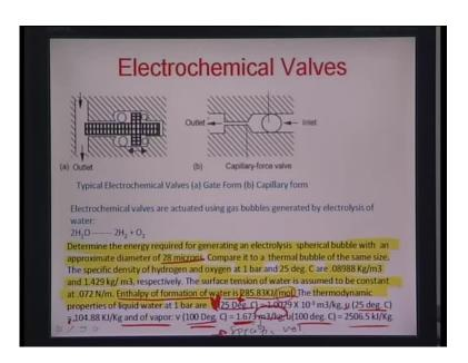
As you see here, specific volume of the water vapor at 100 degrees celsius is given to be 1.673 cube per kg mind you, the thermodynamic state that we have to consider for the bubble to be shaped up is that the water vapor essentially is that 100 degree celsius which is also the boiling point of water. We need to formulate the vapor in order to realize the bubble. Therefore, all specific volumes etcetera which are considered at 100 degrees Celsius.
