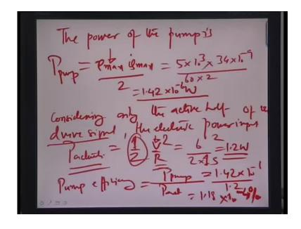
Pumping efficiency is defined earlier is essentially, the power of the pump which we just calculated in the top divided by power of the actuator comes out to be 1.42 times 10 to the power minus 6 by 1.2 which is about 1.18 into 10 to the power of minus 4 percent. So, that is what the pump efficiency is pretty low in this particular case. Thermo pneumatic effects in fact do not really give a lot of efficiency and also, there are awfully slow - the response rate is very slow.
