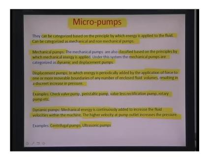
Let us look at a different paradigm altogether which is the world of micro pumps. Essentially, I would like to describe here some of the basic definitions about, what micro pumping is. I would like to categorize into different mechanisms again, there are passive and active micro pumps, there on mechanical non-mechanical pumps essentially. Of course, there up actuation principles or operation principles are based on totally different physical properties or physical effects.
