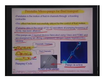
Let us talk about the second mechanism which is peristaltic micro pumps. I would like to show some illustration from one of the research modules that we have developed in our laboratory here. This right here is the example of what a peristaltic pump would typically do micro for fluid transport. Let me just retreat peristalsis in the motion of a travelling contract a fluid due to travelling contract.
