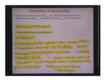
The power of a pump here assuming P max to be the maximum pressure, Q max dash to be the maximum flow rate and assuming that the flow rate starts from 0 and gets this height as the fluid passes through the whole pumping chambers or the pumping system. So, Q max by 2 effectively is the average flow rate. P max into Q dash max by 2 makes the power. We know that the pressure max is also represented by this height max into rho into g, so rho g h max q dash max by 2 is what the pumping power is.
