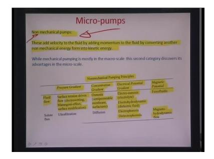
Another is concentration gradient driven mechanisms like osmosis, if you have a charged concentration and you have seen the details of such kind of pumping mechanisms before while doing the chemistry. Essentially, semi-permeable membrane surfactants they would cause this kind of charged double layer along the surface in the solution and diffused layer. This layer can help you to move ahead the flow of fluids is a plug through channels.
