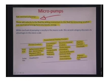
Now, let us describe some of the non-mechanical pumps or types of pumps. Essentially, as I told you before, these really add velocity to the fluid by adding momentum to the fluids by means of converting another non-mechanical energy form into kinetic energy. While mechanical pumping is mostly in the macro scale the second category discovers these advantages of the micro scale.
