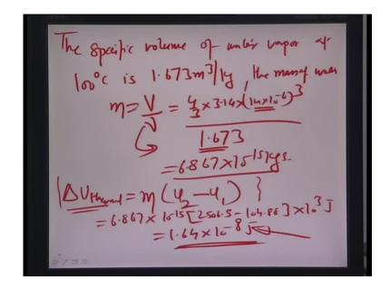
If you may compare this value with electro chemical energy which is needed, it is almost 4 order of magnitudes more in the electro chemical sense is about only 10 to power minus 12 joules, were is in the thermal sense is about 10 to the power minus 8 joules. The thermal means of course, is about 10 to the power 4 times more than the electro chemical means. So, definitely you can understand which one is better or you know more energy efficient process.
