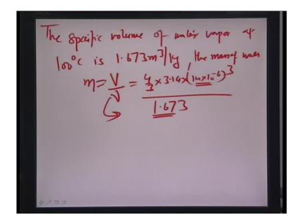
Therefore, if we compare the specific volume of water vapor at 100 degrees celsius and compare that with the mass in order to find out how much amount of thermal energy would be needed to convert that mass to make a thermal bubble. We should be able to
