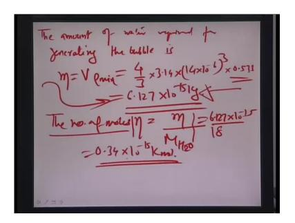
The amount of water required for generating the bubble would be actually equal to this particular specific density times of the volume of the bubble which is needed. This much amount of water if you assume continuity between the 2 phases would have to be essentially decomposed in order to create an equal volume of the gas mixture H 2 and O 2 which would formulate bubble.
