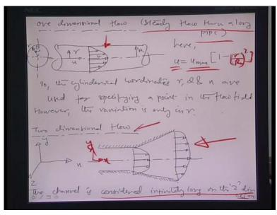
Let us discuss some examples of 1-dimensional flows, especially steady flows through long pipes. You can see here, this really is a variation of velocity profile with respect to the radius r. So, u here is actually equal to u max, which is somewhere in the centre of the pipe, times of 1 minus small r by big radius R square. So, it is varying only on the radius vector. It is symmetric along the angle phi to describe the cylinder it is only varying along the radial direction.
