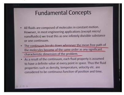
What is important to know that at a more fundamental molecular level? In a fluid, the molecules are not so firmly bound, they are having lesser forces and they are in constant motion with respect to one another. Whatever it is, we still treat the fluid as 1 continuum body, even if the molecules are moving around with respect to another, we still treat as one big continuum, especially in the scales in which we can do bio-sensing or diagnostic.
