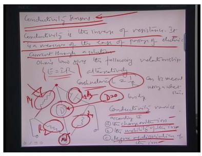
We now shift to briefly to another very interesting area, which is "Conductivity based sensors". So, conductivity is the inverse of resistance, it is a measure of the ease of the passage of electric current through a solution. If you see all the solutions, they can obey Ohm's law. Alternatively, the conductance relation would be a kind of E by L, where 1 by R is equal to the L. So, EL is equal to I, can be what the Ohm's law can be written as in terms of conductivity.
