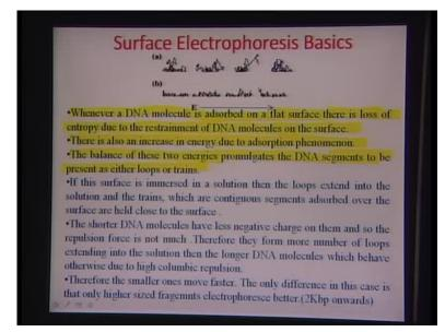
How the surface electrophoresis is done? This is out of a research work done at Benjamin choose group at Stony Brook.
