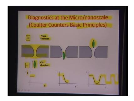
Now, I would like to illustrate another very novel technique of BioMEMS, which BioMEMS has to offer based on various fabrication protocols or various kind of structures and features that can be fabricated using micro systems fabrication technology. So, this is really the diagnostics at Micro Nano scale and is also the basic principle behind Coulter Counters. So, we are talking about a cell counter by the name of Coulter Counter.
