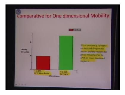
So, this is a study that we did, where we can show that, on a higher energy surface like Silicon dioxide is opposed to a lower energy surface like porous structure, porous matrix made up of Silicon, we have differential mobilities which we report. We are trying to understand the process better, but this is how surface electrophoresis can be done.
