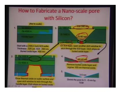
Here, as you see there is an oxide layer of about 400 angstroms. There is a Silicon layer on the top of it of about 2500 angstroms and this whole is assembled onto a handle layer which is a much thicker wafer - a couple of microns; probably couple of 100 microns. Although it is not to scale, it is a 4 inch SOI wafer with this handle layer. Thickness of
