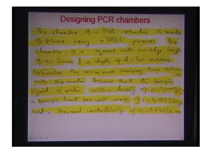
Now let us kind of tried to illustrate that little more with an example. In this particular case as you seeing here, there is a chamber of PCR reactor which is made of silicon using a deep reactive ion etching process. So the chamber is essentially a high aspect ratio chamber used or etched away to using gas plasma the deep reactive ion etching.
