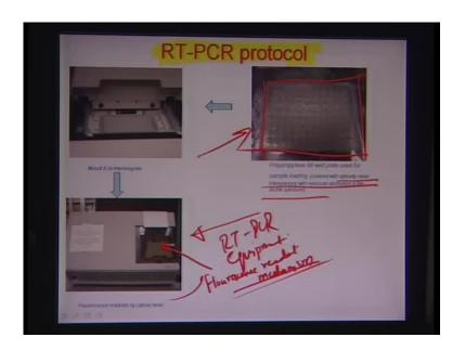
Normally, we do need to read out the fluorescence signal very quickly and for that in especially in the PCR or QPCR reactions we do have a separate reader unit. So essentially there are 2 aspects here; one is there has to be a reader head you can see, this is essentially equipment from strata gene, this is RT-PCR equipment and this right here is also the fluorescence readout mechanism. So what this mechanism is really? It is a set
