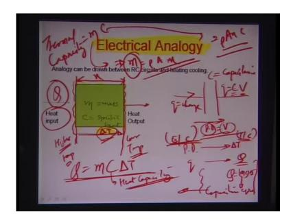
So that is why this particular trend is visible or it comes so. One interesting factor which comes into picture while designing a PCR chips is essentially how you will try to characterize the chips thermally and what you need to do to certain, how much time it would take for the chip to cycle to a certain temperature.
