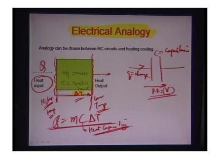
So let us draw the capacitor. This is the capacitor; let us say you have capacitance value equal to c, you have a charge small q which is flowing through this capacitor and essentially there is a potential difference of v here. So what causes the charge really to flows the potential difference here; what causes the heat to here flow is temperature difference here, so it is kind of analogues.
