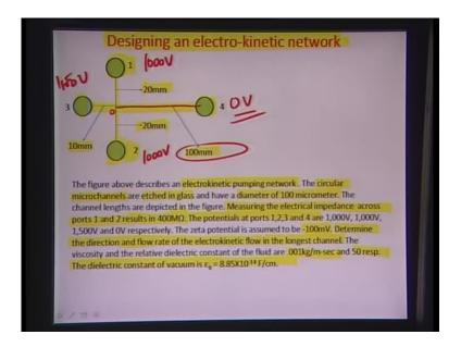
Electrophoresis on the other hand is the motion of charged particles directly in a fluid medium and will be dealing with this a little bit later in more details, but let us look at one illustration here, where we can use this electro kinetic techniques for designing micro pumps.
