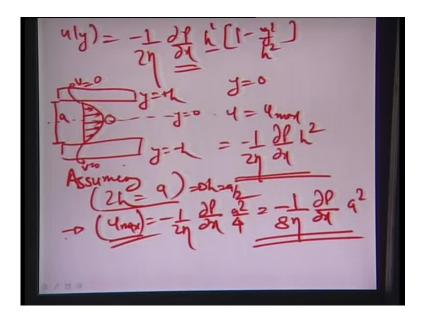
Essentially, the function that we obtained for u in the velocity, in that case was also minus 1 by 2 eta dp by dx h square times of 1 minus y square by h square, where dp by dx essentially is the pressure gradient across the capillary in the x direction. Assume that the two plates are respectively fixed at y equal to plus h and y equal to minus h, the middle of such a plate assembly is really the y equal to 0.
