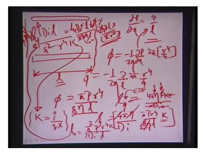
Essentially, this takes the form r square by 4 and we are left with an equation of the type phi equals minus 1 by 2n del p by del x 2 pi times of r 4 by 4. Now, one thing which is of importance here is seen that we consider a channel at the very beginning. If you consider the electro osmotic flow of length 1, you consider the channel of length 1 and if you assume that there is a pressure driven flow in this particular example which is essentially
