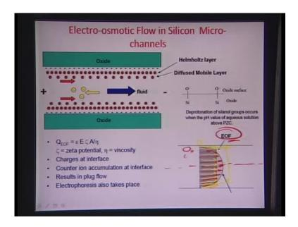
Essentially, if you just compare the other flow profiles which are generated from the EMF and a parabolic flow. If you may recall, in a pressure driven flow the flow profile is something like a parabola of the sort.
