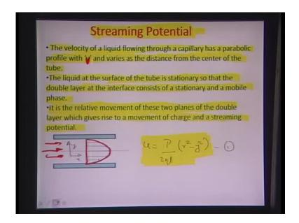
Let us shift our attention to the second electro kinetic phenomena that is the streaming potential. As we talked about before, the velocity of a liquid flowing through a capillary has a parabolic profile with v that varies the distance from the center of the tube to the sides; this is v, the velocity.
