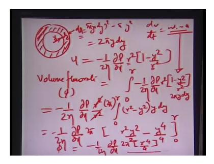
Let us now try to find out the maximum flow rate which would happen because of this function u. So, if you really look at the flow rate, we can assume that in this particular case, there is a circle or there is an annular of area a through which the fluid is emanating out. Add a velocity u which is given by the function shown earlier in terms of the pressure gradient; the square of the y and the square of the distance from the mean plain or y equal to 0, sorry, y equal to plus h and minus h.
