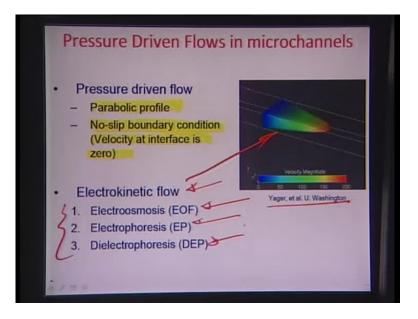
Let us try to summarize that in pressure driven flows essentially, the flow profile is parabolic in nature and there is no slip boundary condition at all, the walls or the edges of such a channel the flow profile pretty much looks something like this here (Refer Slide Time: 37:09).
