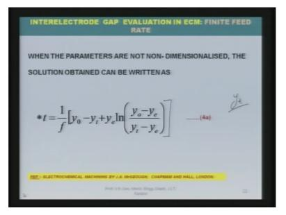
When the parameters are not non-dimensionalised the solution obtained can be written as t is equal to 1 over f within bracket y 0 minus y t plus y e ln y 0 minus y e divided by y t minus y e, this bracket. Now this equation is an implicit equation when you want to evaluate the inter electrode gap y t right. So this equation is given in the book on electrochemical machining by J. A. McGeough published by Chapman and Hall, London.
