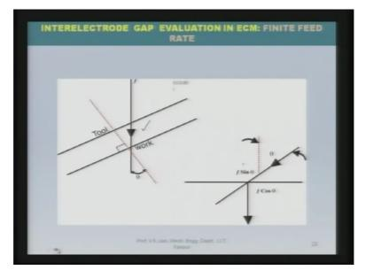
Now most of the time you find that the feed rate is inclined to the surface of the work piece as I can see here in that particular case you have to take the component of the feed rate which is normal to the work piece surface and that becomes f cos theta, so in place of f you have to use f cos theta at appropriate places wherever feed rate term f appears.
