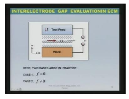
Now in this particular figure we can clearly see that tool is feeding, is being fed downward, there is the flow of the electrolyte in this particular direction with a certain velocity and work piece and tool both are connected to the power supply tool being cathode and work piece being anode. Now here as I have mentioned earlier two cases arise one is the case where feed rate f is equal to 0 and another is the case where feed rate is not equal to 0.
