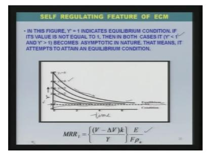
So in this figure which I am going to show, we have seen earlier that whether the inter electrode gap was lower than the equilibrium gap or larger than the equilibrium gap in both the cases inter electrode gap automatically was attempting to attain the equilibrium gap, the same thing which we discussed in the or we saw in the earlier slides is represented here in the form of the graph as you can see here, here is the Y dash and here is the time.
