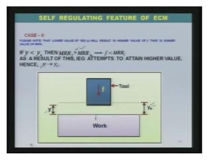
Now case two is the one where inter electrode gap or initial inter electrode gap is less than equilibrium gap, then MRRI that is linear material removal rate will be greater than the linear material removal rate under the equilibrium conditions and f is smaller than MRRI compared to the equilibrium condition.
