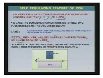
ECM process always attempts to attain an equilibrium gap condition such that y is equal y 0, it always attempts to attain this condition or in other words you can say f is equal to MRRle, here suffix 1 indicates the linear material removal rate and e indicates the linear material removal rate under equilibrium condition.
