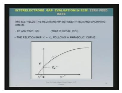
Now this equation yields the relationship between inter electrode gap and machining time, any time t. Now you can see here that as the time t is increasing inter electrode gap is increasing according to the equation which we derive in the earlier slide now here you can see the time t is equal to 0. There is a certain inter electrode gap that is represented by Y0 and that is what we have used in the earlier equation for as the initial condition.
