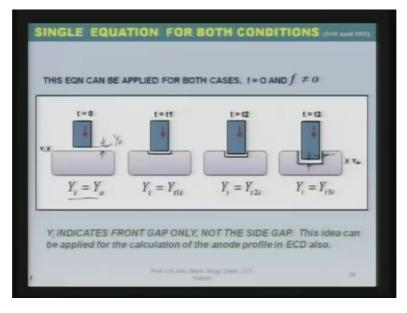
Now what is this Y 0, you know when you are beginning the machining then whatever is the initial inter electrode gap that is Y 0. Now when we deal with the finite element method or other procedure then we in place of Y we can use Y I that is the I S node and Y I is equal to Y 0 and if it is at time T is equal to 0, if time T 1 is there then it becomes Y I is equal to YT1I and so on, as I have shown over here.
