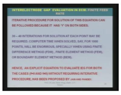
Now iterative procedure for solution of this equation can be followed because it has Y on both sides when you are evolving Y or inter electrode gap with the help of this particular equation, so it takes 30 to 40 iterations for solution at each point. Computer time when solve say for 1000 points will be enormous specially when using finite difference method, finite element method or boundary element method.
