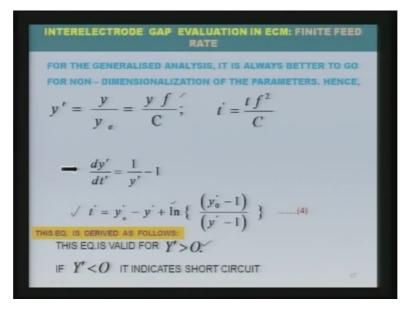
For the generalized analysis it is always better to go for non dimensionalization of the parameter hence here the parameters have been non dimensionalized as you can see y dash is equal to y over y e where y is the inter electrode gap and y e is the inter electrode gap under equilibrium condition and this can be shown is equal to y f over C because we have shown in the earlier slides that y e is equal to C over f.
