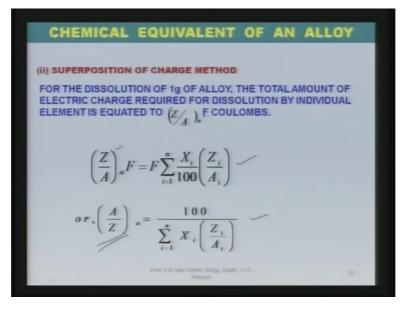
Now super position of charge method, the basic philosophy of super position of charge method is for the dissolution of 1 gram of alloy the total amount of electric charge required for dissolution by individual element is equated to Z over A suffix small a multiplied by F that is the Faraday's constant.
