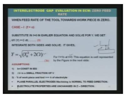
Let us evaluate the inter electrode gap in ECM for zero feed rate, when feed rate of the tool towards the work piece is 0 that means tool is stationary, now substitute in earlier equation f is equal to 0 then we will get that dY as function of Y here is equal to C into dt. Integrate both
