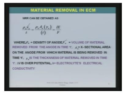
Material removal rate can be obtained as rho a v a over t and volume of anode removed v a, let us see it is given by A a cross-sectional area the inter electrode gap, y a that is the gap divided by t is the time and rho a is the density of the anode material.
