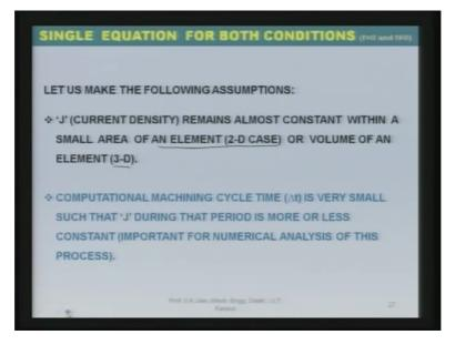
Let us make the following assumptions, J that is the current density remains almost constant within a small area of an element when I say element that means I am talking with reference to the finite difference method or finite element method of 2D problem or volume of an element that means I am talking of 3D problem.
