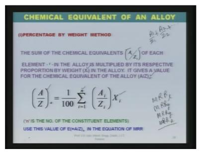
Percentage by weight method, now in this particular case the sum of the chemical equivalent AI divided by ZI, I indicates the IS element maybe written as A1 over Z1 plus A2 over Z2 and so on for different elements of each element I in the alloy is multiplied by its percentage, respective proportion by weight that is XI in the alloy. It gives a value for the chemical equivalent of the alloy that is abbreviated as A over Z with suffix small a.
