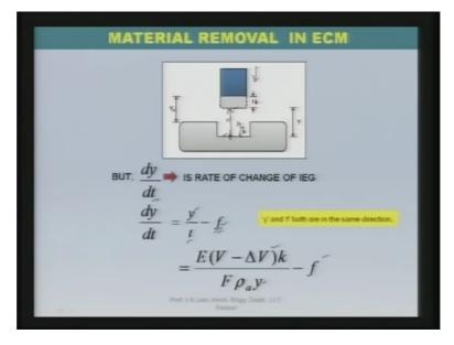
Now dy dt is the rate of change of inter electrode gap, what is this rate of change of inter electrode gap, here let us see we are giving the feed to the tool that is moving downwards and due to the removal of the material the surface of the work piece is also moving downward so both are moving in the same direction.
