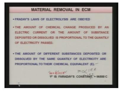
Now we know from all this discussion what are the various factors or parameters that are going to affect the performance of the process. Can, how many of them can be incorporated in the mathematical model with the help of which we are going to evaluate material removal in electrochemical machining, let us see.
