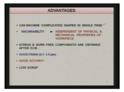
Now let us see in brief what are the various advantages and some of the important application of electrochemical machining process. It can machine complicated shapes in single pass this is very important advantage that very complex shapes say take the case of turbine blades which is 3 dimensional complex shaped component, whole of the turbine blade can be machined in single go or one go and it has really very very complicated shapes.
