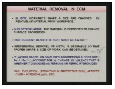
In ECM work piece shape and size are changed by removal of material from the work piece, in electroplating the material deposited to change surface property, so you can see both them are following Faradays laws of electrolysis but one is just reverse of the other.
