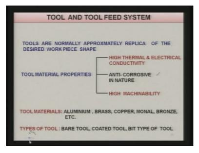
Now another thing is tool and tool feed system this is another sub system which is very important, tools are normally approximately replica of the desired work piece profile this is approximate for exact profile of the hole you have to use proper tooling design technique which I will discuss later on.
