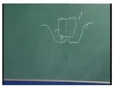
Let us see if vibration is there then suppose this tool is vibrating if the tool is vibrating then the gap that is known as inter electrode gap is also going to change and if inter electrode gap is going to change then material removal rate will keep changing with time and that will create the problem will not get the shape and size of the work piece that you have designed.
