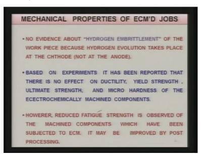
Mechanical properties of the electrochemically machined components or jobs, there are no evidence in the literature available about hydrogen embrittlement of the work piece because hydrogen evolution takes place at the cathode not at the anode, this is very important as I have mentioned earlier also that hydrogen evolution is taking place at the cathode and oxygen evolution is taking place at the anode.
