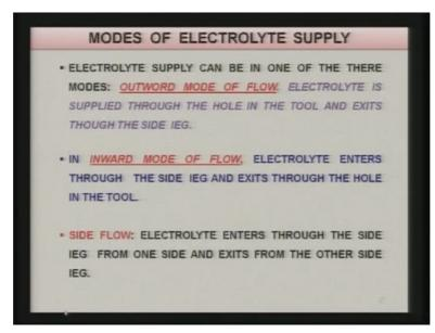
Now modes of electrolyte supply this is something very important, how to supply the electrolyte in the inter electrode gap or the gap between the tool and the work piece. Electrolyte supply can be in one of the three modes as I am going to show with the help of figures also outward mode of flow, electrolyte is supplied through the hole in the tool and it exits to the side inter electrode gap as I will show you the figure in the following slide.
