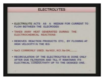
Electrolytes and mechanical properties of electrochemically machined components, electrolyte acts as a medium for the current to flow between the electrodes that I have already mentioned that between the tool and the work piece over here as you can see here is, this is flow of electrolyte so this electrolyte over here makes the medium for the current to flow.
