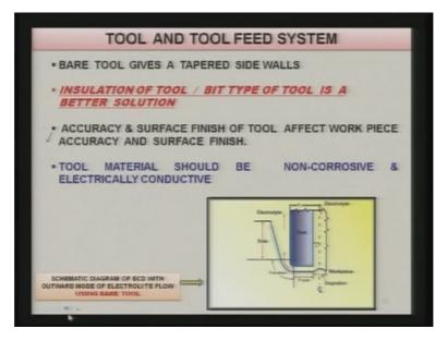
Now next one you can see here bare tool gives a tapered side profile as I have shown to you or side wall, tapered side walls and this gives a clear cut idea here in this particular figure what kind of side walls you are going to get with the help of the bare tool as shown over here. Insulation of the tool or bit type of the tool is a better solution as I have already mentioned.
