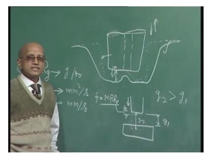
Same way once this has moved this much distance in 1 second then as I mentioned in the last class that if it is like this and this is the initial inter electrode gap in after 1 second the work piece surface has recessed this much so the gap will increase this one, G1 and G2 and G2 is bigger than G1 so to maintain the constant gap you have to feed the tool downward that is why the tool will come over here and this distance by which it is moving downwards should be equal to MRRL.
