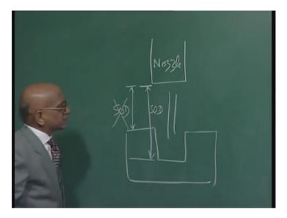
Here one point is to be noted that this stand off distance is not fixed always when the jet is moving inside and it has moved sufficiently below the work piece and here is the say nozzle, this is the nozzle then the stand off distance will be this one, not this one. So it has to be, this is the SOD no and so this has to be measured from the bottom face of the nozzle and the top surface of the work piece where it is removing the material this point should be carefully noted.
