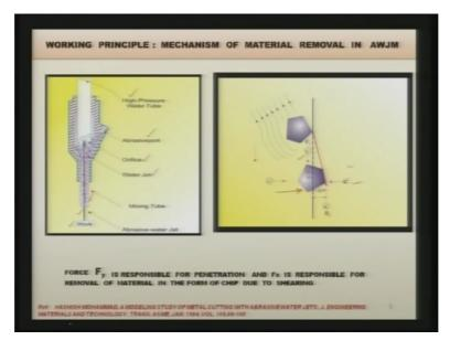
Let us understand the working principle of abrasive water jet machining, it should be water jet machining not C, as you can see here this is the schematic diagram of abrasive water jet cutting system, you can see there is a high power water tube through which the water at very high pressure is supplied and then on this side we have the abrasive port through which abrasive particles are supplied these abrasive particles may be alumina AL2O3, silicon carbide or some other abrasive particles.
