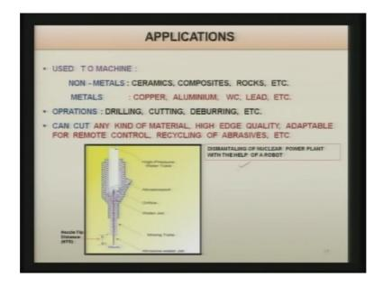
This we have already seen the important thing that you can see here once again is that the distance between the bottom of the nozzle and the top surface of the work piece that is known as nozzle tip distance or it is also called as stand off distance. Now it is used to machine metals as well as non-metals, non-metals materials are like ceramics, composites, rocks, etc.
