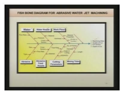
Let us have some parametric analysis of the abrasive water jet machining process, before we discuss it let us first see what are the various parameters involved in abrasive water jet cutting process. Now first of all water is there the pressure of the water and the flow rate of the water both are the parameters for this particular process then there is a water nozzle.
