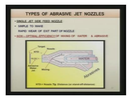
Now abrasive jet nozzles, their various functions of the nozzle in abrasive water jet machining, first one is mixing of abrasive and water jet as we have seen and then forming high velocity jet. Materials of the nozzle are tungsten carbide, boron carbide, sapphire or very hard materials and resistant for wear materials can be used for this purpose.
