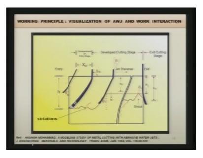
Now what happens really when it starts from one edge to another edge as you can see over here at the entry it cuts it and then starts exiting from the outside or least resistance path and then you can see in the beginning after entry stage it starts tilting or bending at a particular angle and striations in the surface are created as you can clearly see and whenever there is a blind cavity, this kind of the bottom surface is obtained and it is not acceptable in most of the application.
