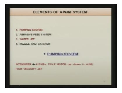
Let us see what are the various elements of abrasive water jet machining system, first one is the pumping system another is the abrasive feed system, water jet, nozzle and pressure of the water as high as 415 mega pascal or so for which the motor around 75 horse power is used. It gives a high velocity jet.
