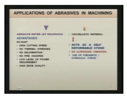
As you can see on the left hand side the improvement on the abrasive jet machining process is the result or as a result of improvement we have what is known as abrasive water jet machining process which has many advantages compared to specifically abrasive jet machining process, there is no dust in the environment, whatever material removal is there, abrasive particles are there all of them are within the water so environment pollution is minimized.
