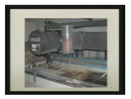
Now you can clearly see various other elements of the abrasive water jet cutting machine, now this is the abrasive tank which is having dry dehumidified abrasive particles, now here is the nozzle and it is going to cut the work piece over there and you can see this is the water tank and this here you are going to place the work piece somewhere here.
