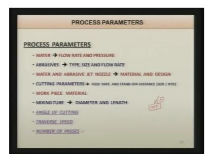
Let us see again the same thing water, we have seen flow rate and pressure, abrasives, types size and flow rate, water and abrasive jet nozzle material and design, cutting parameters are feed rate and stand off distance, work piece material mixing tube angle of cutting, traverse speed and number of passes these three are very important now what angle the jet is hitting the work piece surface.
