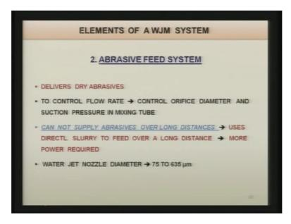
Another is the abrasive feed system we have seen in the figure of the system, abrasive water jet cutting system. It delivers dry abrasive particles to control the flow rate of dry abrasive particles, control the orifice diameter and suction pressure in mixing tube, you can change the
