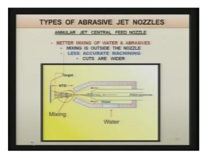
Another one is known as annular jet central feed nozzle, it gives better mixing of water and abrasive but in this particular case mixing is outside the nozzle it is less accurate or it gives less accurate machining as compared to the earlier one in this particular case cuts or the kerf width is higher compared to the earlier one.
