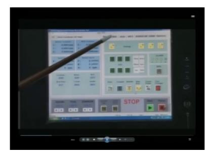
The next window is MDI. MDI is manual data input, this window will help the user to execute a individual block of command, the third window is auto, this is the window where the program is executed. Here there are 4 options given for the user, to open a new file, this is to open a file which is already available in the library, it is to save the file, it is again another option for saving a file in different name.
