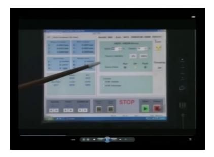
The last option is, this is to set wire EDM parameters. The parameters are the speed and the tension. Another box available is for coolant. Here the dielectric is chosen for the process. So these are the various features of the Control Panel of this machine.
