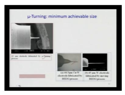
Now this is micro-turning with the help of which a tool is being prepared and this tool can be used for electric discharge micro-machining purposes. 22 micro-meter electrode fabricated by micro-turning process. Here tool is fabricated by the conventional micro-turning and this tool can be used for the purpose of electric discharge micro-drilling operation.
