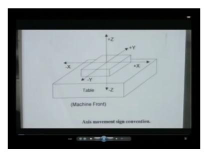
The direction of convention for all 3 axis is shown in a schematic diagram even though all the 3 axis are shown on a single table it is not so in the real machine. In the machine the horizontal table is controlled by y axis whereas the vertical table contains x axis and z axis as well as the rotational axis. The axis of travel for each axis is as follows, the x axis can travel the maximum distance of 200mm.
