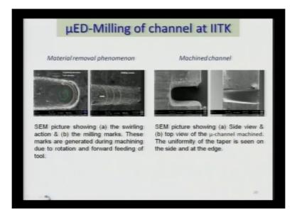
Now you can see SEM picture showing the swirling action and the milling marks these marks are generated during machining due to rotation and forward feeding of the tool. Again machine channel is there these are the SEM pictures.
