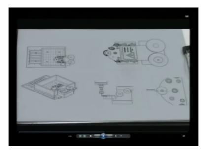
The wire EDG setup is fixed on the horizontal table which is different from the wire EDM setup. Here the wire EDG setup is fixed such that a part of the set up is outside the tank and the part of the set up is inside the tank that is the portion where the machine is going to take place is submerged inside the tank and the portion where the motor is there to guide the rollers is away from the tank.
