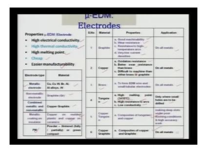
You can prepare micro-EDM electrodes, properties of micro-EDM electrode it should have high electrical conductivity, high thermal conductivity, high melting point, it should be less expensive and manufacturability should be easy, so that you can make the electrodes of different shapes and sizes. Electrode type and material are given here, you can have the metallic electrode where you can use copper, copper tungsten, brass etc. various kinds of the materials.
