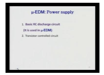
Power supply, normally in electric discharge micro-machining basic RC power circuit is used in the power supply and transistor controlled circuits are normally used for macro EDM but please note that initially it was only the RC circuit which were used in EDM process but later on researchers developed transistor controlled power supply and nowadays in EDM most of the cases you are using transistor controlled circuit for power supply. (Refer Slide Time: 22:26)
