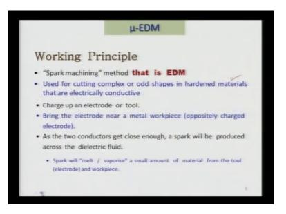
Let us again reiterate in brief the working principle of electric discharge micro-machining. I am saying reiterating deliberately because this principle is the same as the principle of EDM and I have already discussed EDM principle working principle. Now spark machining this was as I mentioned few minutes back. It was initially named as electro-spark machining by Lazarenkos brothers.
