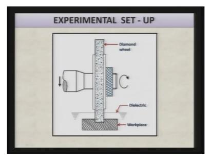
So the grinding wheel setup looks like this that this is the wheel metal bonded grinding wheel or diamond wheel which is rotating and here is the partially the grinding wheel is dipped inside the dielectric and then it is removing the material from the workpiece as you can see here in this particular picture.
