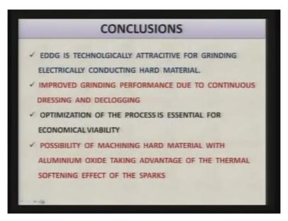
So based on this study certain conclusion have been made, first one is electric discharge diamond grinding is technology attractive for grinding electrically conducting hard materials. The improved grinding performance due to continuous dressing and declogging is obtained.
