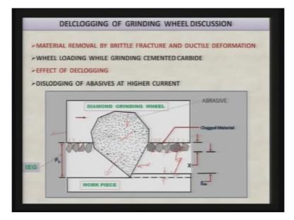
Now declogging of grinding wheel, how does it take place? So that is what we have tried to model it over here, you can see here this is the clogged material which has got deposited between the 2 abrasive particles, there will be another abrasive particle on this side and there will be another abrasive particle the left side. The gap between the bottom phase of the
