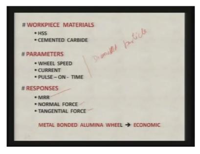
Now workpiece materials can be very hard as we have mentioned earlier also it can be high speed steel, it can be cemented carbide what all these materials should have a certain minimum electrical conductivity, so that they can be a part of electrical circuit, this I had mentioned to you in the earlier lecture. There are various parameters in this particular process as you can see wheel speed is there, current is there, pulse on time is there. I have not
