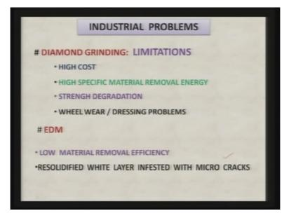
With diamond grinding which is quite common in various types of high-tech industries, there are certain limitations because of which this process has limited applications. First thing is diamond grinding, initial equipment itself is very expensive and the cost of the grinding wheel is also quite high. Then high specific material removal energy requirement is there that means the energy requirement per unit volume of material remover is much higher compared to other machining processes.
