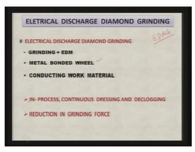
Now electric discharge diamond grinding as I have mentioned that diamond particles abrasive part diamond particles are used as the abrasive particles, now there is...there was another process in the earlier slide I called it as EDAG electric discharge abrasive grinding. Here in
