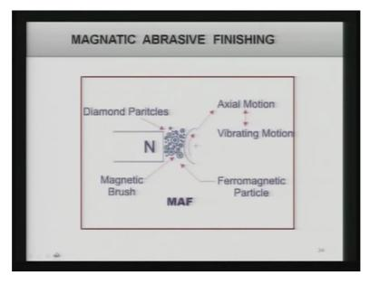
Now there is another process known as magnetic abrasive finishing we can understand this, in this particular process what you have is the diamond particles which have been centered with the ferromagnetic particle and once this ceramic particles have been centered with the ferromagnetic particle they form what is known as magnetic abrasive particles and that is shown over here.
