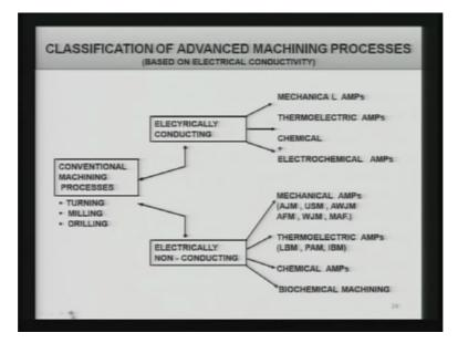
So you can have the classification of the advanced machining processes based on type of the work piece material as I have already mentioned that conventional machining processes which includes turning, milling, drilling, etc. Electrically conducting materials can be machined with the help of, electrically conducting materials can be machined by mechanical advanced machining processes, thermoelectric advanced machining processes, chemical and electrochemical machining processes.
