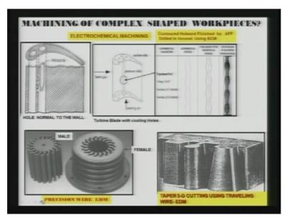
Here we can see some of the very important examples where by which we can say that yes we need some new type of machining processes for solving these problems. Just let us see this example work, here they are the two holes, hole 1 and hole 2 in a turbine blade, now suppose we want the hole which is perpendicular to the access of these holes as you can see here one hole is needed here another hole is needed here third is needed here.
