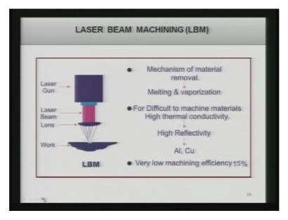
Now in laser beam machining process what you are doing is you are concentrating the laser light on a very small area and in that small area the heat intensity is so high that the it may be as high as that at the sun and you are able to machine or remove material from the work piece of having any hardness and very high temperature resistance material RA can be machined by this particular process very easily.
