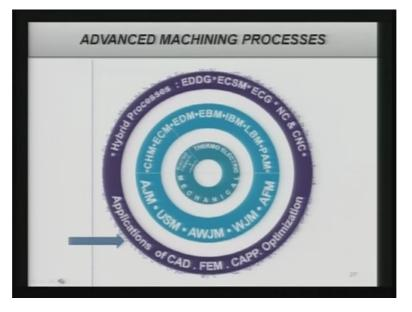
Now this is the Advanced Machining Circle where various kind of the machining processes are shown as you can see here these are the mechanical advanced machining processes, thermoelectric advanced machining processes, electrochemical and chemical advanced machining processes. Now if you see next circle, here they have been again classified like according to the classification which I have already discussed.
