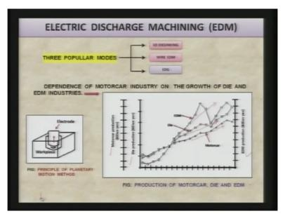
Now this is the slide very interesting slide which I should have shown you in the beginning itself, you can see here production of motor car die and EDM process. EDM as I mentioned, EDM process is very commonly used the purpose of die syncing or in aerospace industries or auto mobile industries or other industries as well. Now one thing is that the dependence of motorcar industry on the growth of die and EDM industries because EDM is very commonly used for die making.
