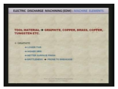
Now tool materials which are commonly used they include graphite, copper, brass, tungsten, et cetera. Graphite has low tool wear rate, high material removal rate, better surface finish but it is brittle in nature, so it is prone to breakage this is the important weakness or this is the weakness of the graphite as the tool material in EDM process, even then this is also commonly used tool material.
