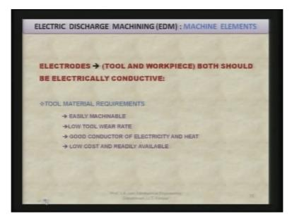
Now electrodes, we have 2 electrodes 1 is the tool another is the workpiece, tool may be mostly it is cathode but sometimes it may be anode also and workpiece mostly it is anode, sometimes it may be cathode also and both should be electrically conducted only then you can have the EDM process and operation. Anyone of them if it is electrically non-conducting then it cannot form a part of the electrical circuit and then EDM process will not take place.
