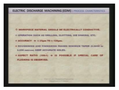
I have already mentioned that workpiece material should be electrically conducted otherwise it cannot be machined by EDM process and operations such as drilling, slotting, die sinking, et cetera can be easily performed using EDM process. The accuracy that you can obtain by this particular process is plus minus 25 micron 2 plus minus 120 micron. Roughing and finishing passes minimise taper and you can make deep accurate holes. The taper can lie somewhere 0.005 to 0.050 millimetre per centimetre.
