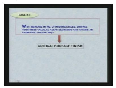
Second issue which is important in case of magnetic abrasive finishing is with increase in number of finishing cycles, surface roughness value Ra keeps decreasing and attains an asymptotic nature. The question arises and as a lay man or in general way if you keep increasing finishing time it is Ra value should keep decreasing but after a certain number of
