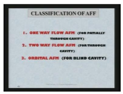
This work on this particular area was started by the extruded home company of USA. There are different models of this particular process as you can see here there are 3 types of the abrasive flow finishing process one is one-way flow abrasive flow finishing process which is applicable for partially through cavity and there is two-way flow abrasive flow machining
