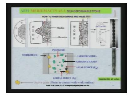
Now let us see medium in abrasive flow finishing process or abrasive flow machining process, the medium in AFM process acts as a self-deformable stone, how to finish different kind of the shape which are shown in this particular slide is really a problem. Here you can see the octagonal hole shape which you cannot finish by normal finishing processes even with MAF you cannot apply that one here.
