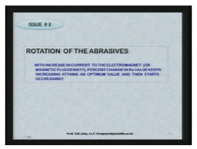
3<sup>rd</sup> issue related to magnetic abrasive finishing which is applicable to other of processes which I just mentioned like abrasive flow finishing and magnetorheological abrasive flow
