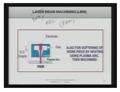
There is another process called, this is the Plasma Arc Machining not Laser Beam Machining so you can correct it this is plasma arc machining, PAM. Now in this particular as you see here you have the gas which is coming in and it is connected to the electrode which is connected to the negative terminal and here is the work piece which is connected to the positive terminal and very high potential is applied.
