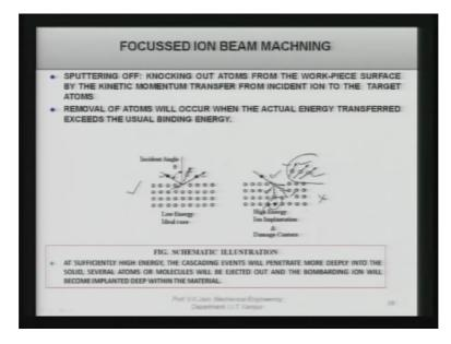
Now focused ion beam, here sputtering off or knocking out of atoms from the work piece surface by the kinetic momentum transfer from incident ion to the target atoms takes place. I will explain it here with the help of the figure as you can see this is the ion of some gas is coming and hitting the top surface of the work piece and you can see here it has displaced the atom from this particular point and you can see here is that atom and here is the ion.
