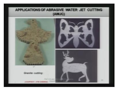
Now you can see the examples of the applications of these processes specifically abrasive water jet machining process, here a granite cutting has been done and you can see very beautiful shape has been formed. Again here there is another application of the abrasive water jet machining and there is a third application of abrasive water jet machining, these photographs are taken from Indian Institute of Technology, Madras, Chennai.
