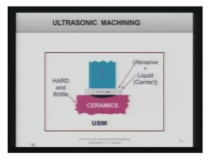
Now working principle of some other advanced machining processes, now there is another advanced machining process called ultrasonic machining process. Now in this ultrasonic machining here you have the tool which is vibrating at ultrasonic frequency that means near or more than 20000 hertz, means 20000 times per second it is vibrating with a certain amplitude of vibration and here if you see here there is a slurry which consists of liquid say water and abrasive particles.
