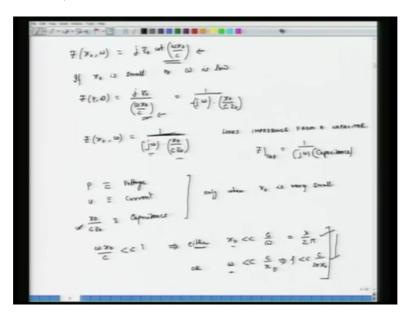
So once again I will write down Z of x not, so suppose the total length of the tube is x not, so then Z at x not omega equals j Z not co-tangent omega x not over c and if x not is small or omega is low, so either my length of the tube can be extremely short or my omega can be extremely low then in that case Z x not omega equals, so then this term can be approximated as j Z not over omega x not over c or I can rewrite this as 1 over minus j omega times x not over c Z not.
