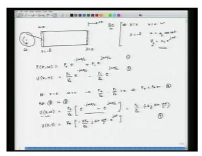
So today we will do a similar example but in this case we will have a velocity boundary condition at the open end of the tube. So once again we have a closed tube and that is my rigid end, x equals 0 at the closed end of the tube and at the open end x equals minus 1. Further I have a piston which moves in and out in a frictionless way and that piston is being driven by a rotating member which is spin on a disk like this.
