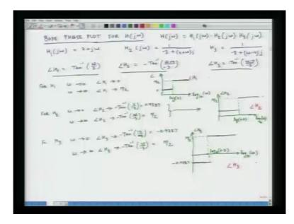
So now our objective is to develop a bode phase plot. A bode phase plot for H of j omega, so once again my H of j omega is a product of H1 j omega times H2 j omega times H 3 of j omega and once again for purposes of clarity I am going to rewrite the functions for H1, it is 2 plus j omega for H2 it is 1 over minus 3 plus 4 plus omega times j and for H 3 it is 1 over minus 3 plus omega minus 4 j.
