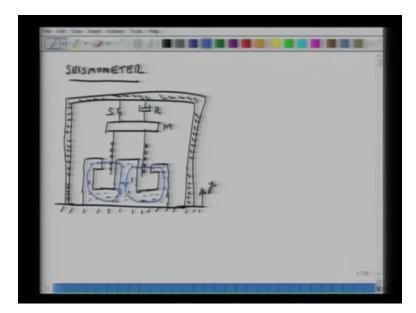
Let us consider if this is a structure and it is rigidly connected to ground and let say the vibrations in the ground are y the construction of seismometer is something like this so I have a motor structure and within this motor structure I have a voice coil.
