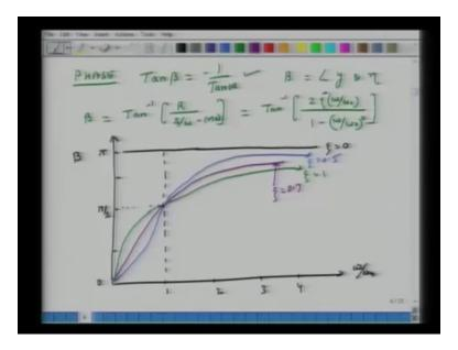
Given that we define this term beta equals phase difference between y and eta. So eta so beta equals tan inverse r over s divided by omega minus m excuse me times omega and this is tan inverse to eta omega over omega not divided by one minus omega over omega not the entire
