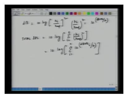
So we know that db equals 10 log pi over p ref right, so pi over p ref equals 10 to the power of db spl over 10, so if I have a bunch of decibel sources then total spl I can write is 10 log summation of pi over p ref square equals 10 log so this is fairly straight forward right.
