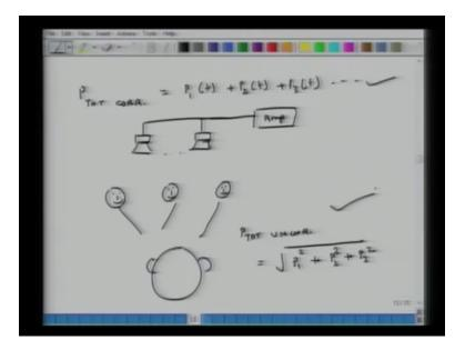
So you have a co related sound p total co related is essentially p one times t plus p two times t plus p three times t and so on and so forth a good example of this could be I have one speaker I have another speaker and both are having the same frequency response curves and they are being fed from the same amplifier the same signal and also the distance between these two is not significantly large.
