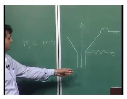
So what that means is that this entire structure and when you draw the mode shape you will see that finite element will predict that this entire thing moves up and down in the modal analysis. That is the pistonic rigid body motion that is fine and may be some other mode M 2 what it will do is that it starts instead of moving like that the cone also has a propensity in the structure to do this, right?
