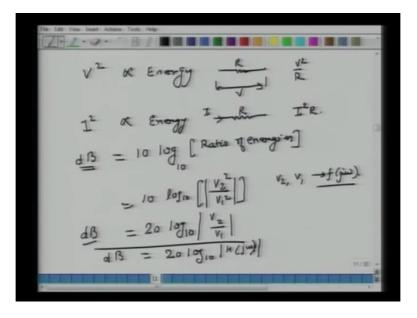
V Square which is square of voltage is essentially proportional to energy. For instance across a resistance if I have voltage V and the energy dissipated is V over R. Similarly I square is again proportional to energy in a general sense, again if I have the example of a resistance and the current going through it is I find the value of resistance is R and energy dissipated or power dissipated is I square R.
