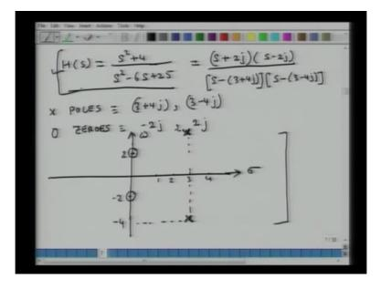
We will do another example and in this case the transfer function is HS equals S square plus 4 over S square minus 6 S plus 25, so I can decompose the numerator into its roots, so that is S plus 2j times S minus 2j and then the denominator is S minus 3 plus 4j times S minus 3 minus 4j. So my poles which are designated as X are roots of the denominator, so it is 3 plus 4j and the other pole is 3 minus 4j and my zeroes designated as O are minus 2j and 2j.
