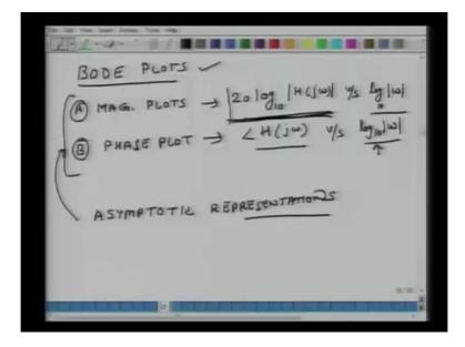
So they can be 2 type of bode plots, one is magnitude plot and this is basically a plot of 20 logarithm on based 10 magnitude of H j omega was on the horizontal axis we have log of omega, again it is a log10 and the second bode plot is a phase plot and here we are plotting
