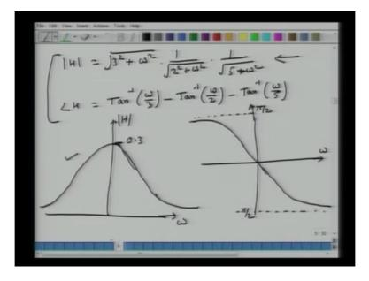
So in this case the phase of, so again the magnitude of H is basically the magnitude of H1 and freshman is 3 plus omega j, so magnitude of H1 is 3 square plus omega square times magnitude of H2, so I will write down that times 1 over 2 square plus omega square the whole thing under square root and then similarly I have magnitude to write down magnitude of H3. So it is 1 over square root of 5 square plus omega square.
