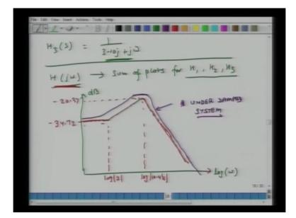
So I have constructed the plot for H2 and H3 and I have constructed the plot for H1 j omega. So my next step is to construct a final plot. So H of j omega which is essentially a sum of plots for H1, H2, H3 so if I have construct a bode magnitude plot for H it is essentially a sum of bode magnitude plots for H1, H2 and H3 and that curve looks something like this. So initially I have a horizontal line then I have an upward sloping segment and then I have a downward sloping segment.
