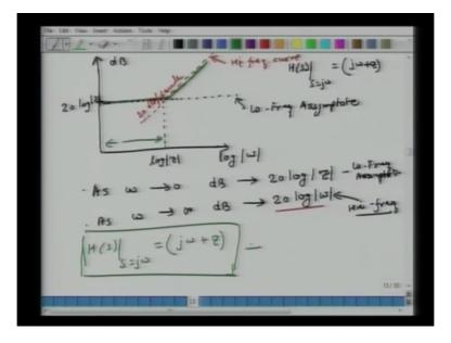
So I will plot these, so my vertical axis as I had said is on a decibel scale, my horizontal axis is on a log scale, so I am plotting log omega on the horizontal scale, on the vertical scale I am plotting decibels and I am plotting decibels for the transfer function HS as S equals j omega equals j omega plus Z, we had seen that as omega goes to 0 the value of dB tends to 20 log Z and as omega goes to infinity the value of dB goes to 20 log omega.
