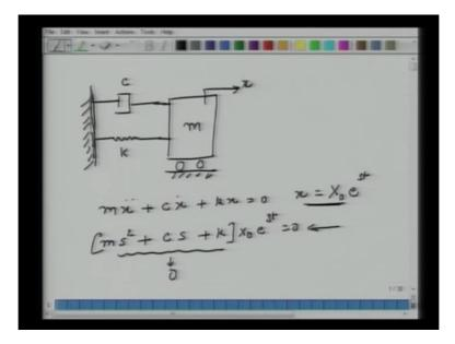
So let us consider a dashboard and then I also have a spring, so the dashboard viscosity is C spring constant or the stiffness member is K and both these elements they are connected to a rigid body mass which can move on a frictionless surface. So now let us assume that I am trying to perturb this by a small displacement x. So from previous classes we know that in such a situation the system is governed by differential equation of this type mx double dot
