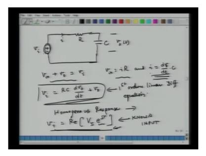
So we have drawn this circuit Vi and Vnot, so input was Vi and output which we were trying to find out is Vnot and we developed a ratio Vnot over Vi is this much.
