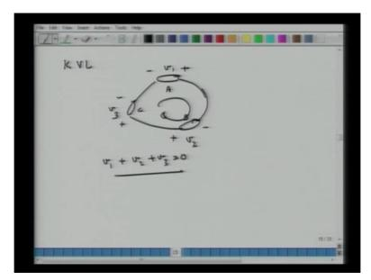
Another law developed by Kirchhoff's is called KVL or Kirchhoff's voltage law. So I have a loop, a close loop of electrical circuit let say around this element I have voltage of V1, here I have voltage of V2 and here I have these are 3 element ABC and here I have a voltage difference of V3 then Kirchhoff's voltage law says that if I go around a loop then it's V1 plus V2 plus with 3 equals 0. So we will be using these notions also in acoustics circuit, so that's why it's good to recapitulate.
