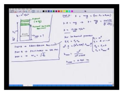
So this is my cylinder and in this cylinder I have a piston, the initial height of the piston, so I call it h initial is 1 meter and of course gravity is acting in the vertical direction downwards. Right now when the height is 1 meter the piston is not released and at this point of time the pressure outside is 10 to the power of 5 Newton's per square meter. So pressure outside then also in the inside is 10 to the power of 5 newtons per meter square.
