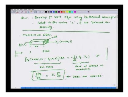
So we have developed the force balance equation or the momentum equation and we have developed the equation which dictates how the gas is behave in this case and this equation is called equation A and this equation as B, what we find is that the material constitutive behaviour has changed because here gamma does not appear because we have isothermal process. (Refer Slide Time: 17:03)
