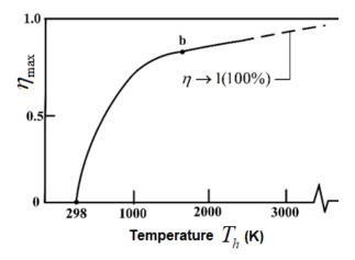
So, if you plot the efficiency versus  $T_h$  for a given  $T_c$ , then we can get a curve like this which says that, with increase in the  $T_h$  that means, with increase in the heat addition, Carnot cycle efficiency goes up. Now we are going to apply same logic for the Rankine cycles. So, for that purpose we need two important observations because the Rankine cycle consists of components like boiler which operates at higher pressure and condenser which operates at lower pressure.
