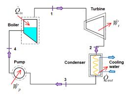
This is state 1. So, if you recall this ideal Rankine cycle the circuit diagrams saturated steam enters at 8MPa and saturated liquid leaves the condenser at 0.008MPa.
