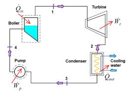
Now, next problem which imposes the component efficiency. So, the component efficiency when it is introduced, we say the turbine and pump operate at 88 percent efficiency. Now, for that process how the cycle is going to be modified we can redraw the cycle in a manner that we can introduce the component efficiency.
