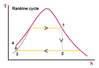
So, in this T-s diagram we are going to locate all these points. So, process 1-2 is turbine, 2-3 is condenser, 3-4 is pump and 4-1 is the boiler and vapor pressure in turbine process 1-2 is at  $p_1 = 8$ MPa and in condenser process 2-3, it is at  $p_3 = 0.008$ MPa.
