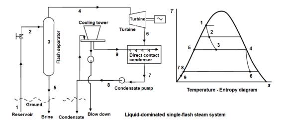
So, we have liquid here, we have vapor here. And it is given in the question that we have an instrument which is called as cyclone separator or flash separator and that flash separator separates the brine that enters into the circuit and that separation happens at point 3. So, it is said in the question that the geothermal system uses a hot water reservoir it contains water at 240°C and 11 bar.
