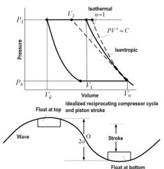
effectively we have the stroke of the piston. So, initially we have atmospheric air conditions at  $p_0 \& V_0$ . So, atmospheric air gets compressed during the compression stroke of the piston and the final volume becomes  $V_1$ . Now, this compression is called as a polytropic compression, so  $pV^n = C$ .
