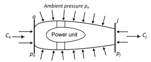
So, in this case if you take this entire unit as a single entity we see that air enters to the duct at a velocity  $C_a$ . We call this as intake air velocity. And combustion products leaves at velocity  $C_j$  which is called as exit jet velocity. So, we have two velocities, one is air velocity other is jet velocity. So,  $mC_a$  stands as intake momentum or drag and drag means it is the force that being experienced by this duct.
