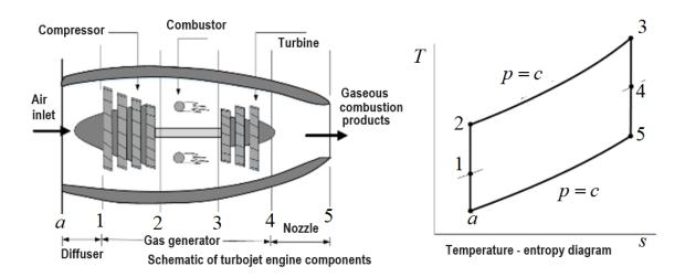
So, if you look at this particular figure, there are three sections shown that are diffuser, gas generator and nozzle. And some important events happen at various locations and locations are noted as a 1, 2, 3, 4 and 5. So, these numbers essentially says that when air enters into
