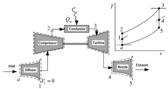
One such simple cycle is the turbojet cycle and we call this as a turbojet engine. So, an ideal turbojet engine has five basic components diffuser, compressor, combustor, turbine and nozzle.
