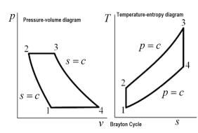
diagrams we also have isentropic compression 1-2, constant pressure heat addition 2-3, isentropic expansion in the turbine 3-4 and constant pressure heat rejection process 4-1. So, here we have net work output denoted by difference in the turbine work and compressor work and heat addition that is taken place from the fuel in the combustion chamber that is  $Q_{in}$  and  $Q_{out}$  is heat rejected in a heat exchanger.
