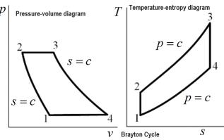
is  $Q_{out}$ . So, this is what we see in the pressure volume diagram. Similarly, 1- 2 is isentropic process in the compressor, 2- 3 is the heat addition process in the combustion chamber, 3 - 4 is the expansion process in the turbine and 4 - 1 is the heat rejection process at constant pressure.
