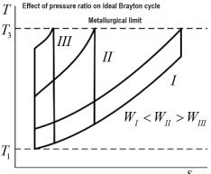
This particular plot of temperature entropy diagram shows the effect of pressure ratio in the Brayton cycles. So, basically  $T_3$  is the maximum temperature. The
