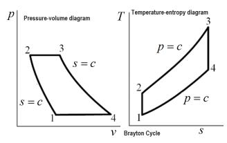
So, here we say s = C that means entropy is constant & here p = C, pressure is equal to constant. So, basically we have  $Q_{in}$  and we have  $\dot{W_C}$  that enters into the system.  $\dot{W_T}$ , is power that is being produced. So, with this notations the data that is given is as follows.
