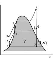
to 7. So, thereby pressure as well as temperature is increased in a regenerative cycle with open feed water heater arrangement. So, this is all about the thermodynamic aspects.
