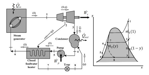
desired pressures. And here main intention is that both the steam that is the steam that is tapped from the turbine and the water that enters from the pump they do not mix. So, that is the thing why you call this as a close type feed water system. So, here the concept, which you have already discussed so far, goes like, if you say 1 unit of steam enters into the first stage of turbine that is HP turbine at state 2 and we take y unit of steam and rest
