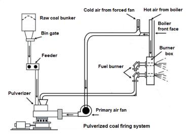
enters into the fuel burner. So, basically to push this fuel or this coal into the fuel burner, we require a fan that pushes these things here then it enters to the burner box and coal firing starts.
