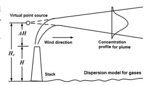
this is nothing, but your first objective that is assisting the fan to overcome the pressure losses. If you use the stack ultimately we will be trying to reduce the fan power. But the second main important objective of the stack is the dispersion of flue gases. The dispersion of gases in the atmosphere is defined as the movement of flue gases horizontally as well as vertically and their dilution by the atmosphere.
