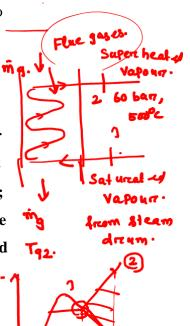
So, the first problem talks about a modern steam generator unit in which super heater coil has to be incorporated. Its dimensions are given like internal diameter 52 mm and thickness 5 mm exit condition of the steams are 60 bar and 500°C, flow velocity 15 m/s mass flow rate 75 kg/s. Due to material restrictions, the heat flux in the coil should not exceed 150 kW/m<sup>2</sup>.
