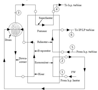
heater and air pre-heater. So, our main goal in this lecture is that we will be mainly focusing on the super heater part. Before you go for those super heater component, let us think about in a broad sense what do you mean by heat absorption in the water tube boilers.
