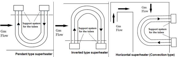
steam flow rate, user needs to have a flat type of curve where the temperature remains to be flat. So, for that case the combined super heaters are most beneficial and they are called pedant type super heaters. So, that is the main advantage.
