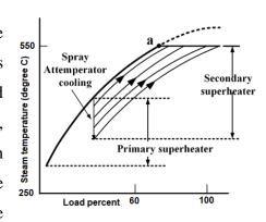
range of temperatures. So, attemperation is a method of reduction of steam temperature, which is done by two methods, one is surface attemperator & the other is spray or direct contact type attemperator.
