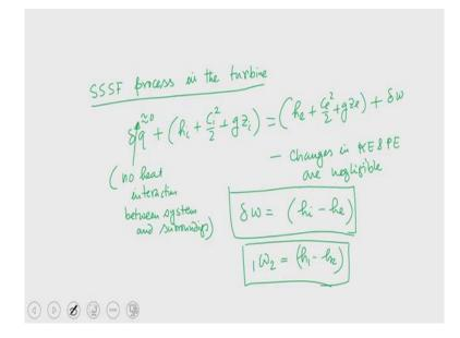
Steady state steady flow process in the turbine
