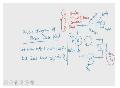
So, we try to discuss today the block diagram of steam power plant. So, I am trying to just represent not all components but the major components which are used in the power plant. So, the first component is boiler and next important component is turbine. And I would like to discuss a few important issues before I go to discuss about the rest of the components of this particular system.
