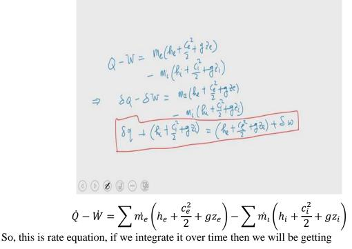
$$Q - W = m_e \left( h_e + \frac{c_e^2}{2} + gz_e \right) - m_i \left( h_i + \frac{c_i^2}{2} + gz_i \right)$$
