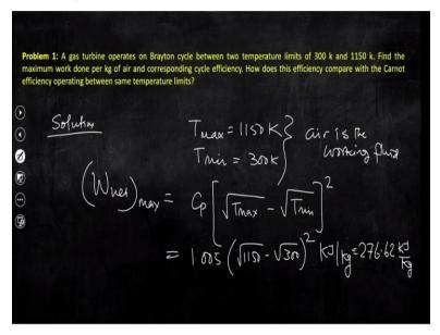
So, this is the first problem, let me read out the problem statement first. A gas turbine unit or cycle operates on Brayton cycle between two temperature limits of 300 K and 150 K. Find the maximum work done per kg of air and corresponding cycle efficiency. Then we need to show how does this efficiency compare with the Carnot efficiency operating between same temperature limits.
