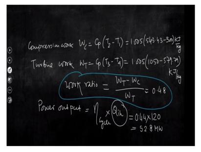
Then next we can calculate the compression work & turbine work.
