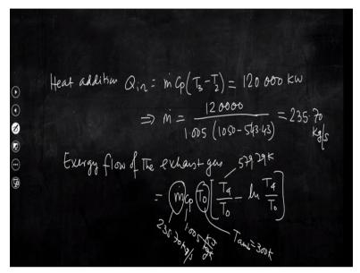
Heat addition,  $Q_{in} = \dot{m}C_p(T_3 - T_2)$
