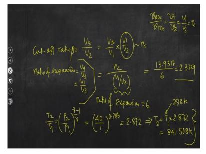
$$Cut - off \ ratio, \beta = \frac{V_3}{V_2} = \frac{V_3}{V_1} \times \frac{V_1}{V_2} = \frac{V_3}{V_1} \times r_c$$
