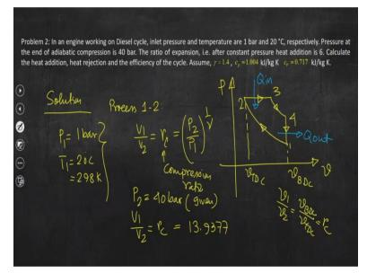
So, then we have to move to the next problem that is this problem is taken from the CI engine. What is this problem statement? Let me read out once again in an engine working on diesel cycles you can understand this is the CI engine because we need to analyze the performance of this engine by considering an air standard cycle and that cycle is diesel cycle. Typically performance of compression ignition engines is analyzed based on the diesel cycle.
