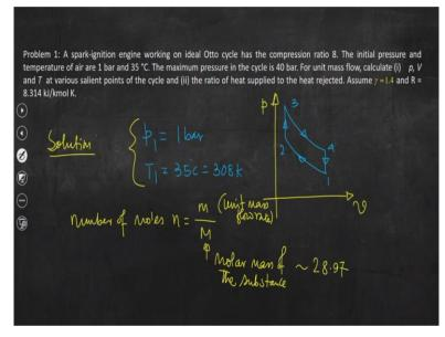
So, this is the first problem let me read out the statement of the problem first. A spark ignition engine working on ideal Otto cycle has the compression ratio 8. So, it is telling that the engine is a SI engine and it is working on ideal Otto cycle because we have discussed that we need to compare several processes using an air standard cycle and for the SI engines we considered Otto cycle for this comparison.
