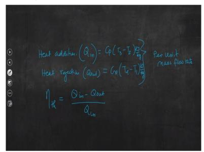
So, next part is heat addition, see in the previous problem we could write heat addition per unit mass of flow of the walking substance that is Cv multiplied with T3 - T2, but here it would be
