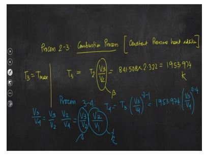
So, I am writing here process 2 to 3 that is the constant pressure heat addition combustion process.
