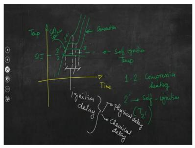
So, we have discussed about the knock which may develop that is nothing but abrupt pressure rise alongside the generation or development of an audible noise. And that may happen if the self ignition temperature of the fuel which is being supplied to SI engine is really less.
