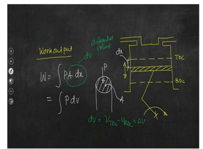
So, if we draw the schematic, this is the top dead center and this is the bottom dead center and piston is having reciprocating motion between these two centers TDC and BDC. So, we need to induct air if it is a CI engine or airflow mixture through this intake manifold to the engine cylinder and piston is having movement between these two stops and we have identified several Strokes.
