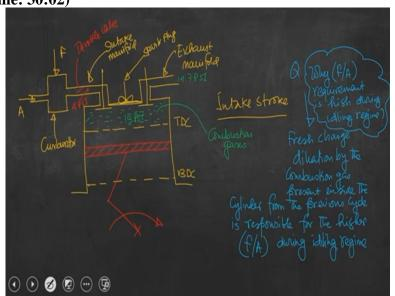
So if we draw the schematic, so this is carburetor and this is intake manifold, intake valve, this is exhaust valve, this is top dead center, this is bottom dead center, this is exhaust manifold, this is spark plug and this is carburetor, this is fuel supply this is air supply. So let us now recall the strokes.
