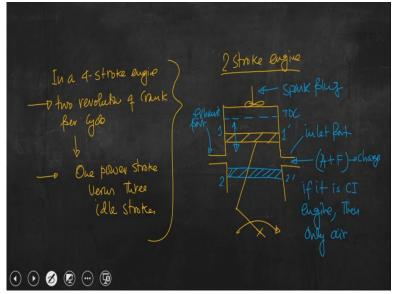
So what we can understand from this analysis is that in a 4 stroke engine, we have identified 2 revolution of crank per cycle and we have also identified 1 power stroke versus 3 idle strokes. Now question is what about 2 stroke engine, you can understand that only 2 strokes will be there.
