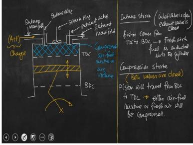
So if we try to draw the schematic of an internal combustion engine, so this is top dead center. And if we say this is the piston and this piston connected to this crank using this connecting rod. And piston is having to and fro movement inside the cylinder, so this is engine cylinder, say this is the bottom dead center. So we had seen this is intake manifold, this is intake valve.
