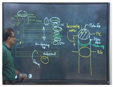
So I have tried to represent a schematic of the internal combustion engine essentially to show you the nomenclature or rather to identify several parts, because depicting this arrangement we have understood that combustion should takes place internally. It is because of this combustion the amount of heat that will be leverated that heat should be utilized to have the reciprocating moment of the piston. So, this is engine cylinder and inside the cylinder we can see that is piston.
