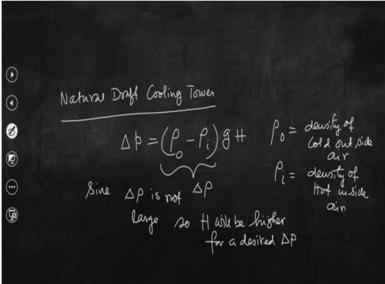
So in this particular classification natural draft cooling tower as I said you that the pressure difference is needed to make the flow occur; so, that pressure difference is due to the density difference.
