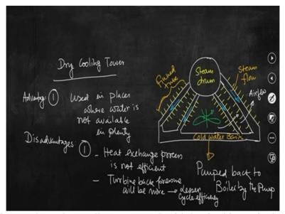
So now let us discuss about dry cooling tower as I said that in this particular type 2 different streams do not mix together instead heat transfer or heat exchange you will takes place while one stream is passing through the tube or tubes and another stream will pass over the tubes. So if we try to understand the mechanism of this heat transfer it would be you know convenient if we discuss it with a schematic.
