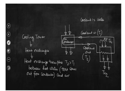
So, just if we draw this is the condenser and so this is coolant in and this is coolant out. So here stream is flowing over the tubes through which that coolant is circulated and coolant is water. Now since the temperature of water at the exit here is  $T_2$  and certainly  $T_2$  is greater than  $T_1$ . And that was the purpose to reduce this temperature of stream so that stream will be condensed.
