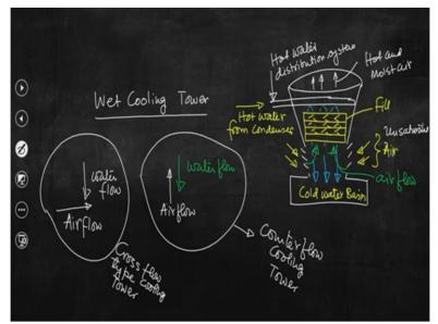
So, wet type cooling tower type, 2 different streams that is hot water and ambient air will mix together, let us now draw the schematic depiction of this particular type. Then we shall discuss about the internal arrangement and also the flow processes.
