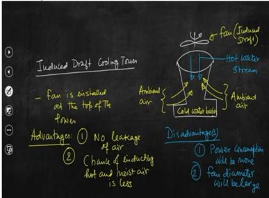
Now coming to the induced draft cooling tower, if we again try to draw the schematic, so this is hot water stream and ambient air and that is cold water basin. We can see this is the fan and
