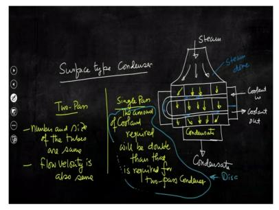
Now let us look into to the surface type heat exchanger or surface type condenser as I said you that the condenser is a type of heat exchanger. So, it is a surface type heat exchanger. Now if we try to recall in surface type condenser because of its name, it is designed in such a way that 2 streams will not mix together that means 2 streams will be exchanging heat while they are passing through the condenser without getting mixed.
