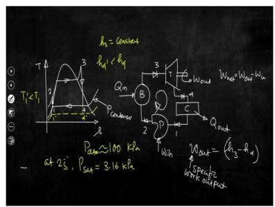
So, we have drawn the steam power plant schematically in the slide. We will see that condenser play an important role. So, there is a turbine from which we get work output. Then there is the
