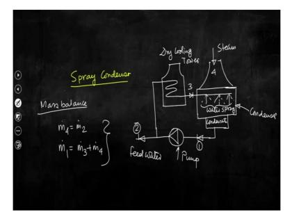
Now let us discuss about one particular direct type condenser just for the sake of understanding how this particular type works. So, there are different types available in the category of direct type. So, one particular type is spray condenser. So, now let us try to draw the schematic. There is condenser, pump and dry cooling tower drawn in the schematic.
