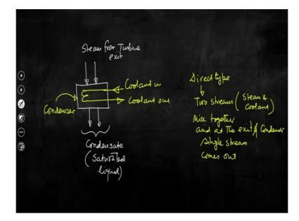
So, let us try to draw this unit again. To this condenser steam comes out from the turbine exit and we will be getting condensate saturated liquid at the exit of the condenser. Because we would like to use pump so this is the saturated liquid. Now this process is basically a heat exchanging process. So, that means we need to circulate coolant and the coolant in and coolant out has been marked in the schematic.
