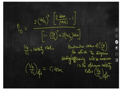
So, we had discussed about this particular velocity ratio in the context of impulse turbine. So, again we can see that the diagram efficiency or blading efficiency of the reaction turbine can also be expressed in terms of velocity ratio. Now try to understand that there is a particular value of this ratio for which the diagram efficiency will be maximum and to obtain that optimum velocity ratio we need to differentiate  $\eta_D$  with respect to the velocity ratio and equate it to zero.
