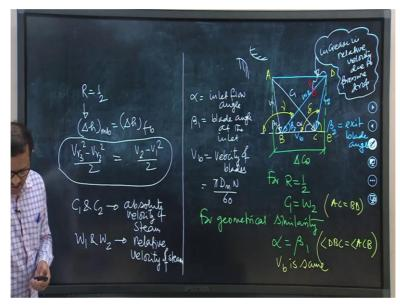
So, if we try to draw the velocity triangle for this particular case that is  $R = \frac{1}{2}$  then what we can understand for this particular case is that the enthalpy drop of steam while passing through the moving blades is equal to enthalpy drop of stream passing through the nozzles or fixed blades.
