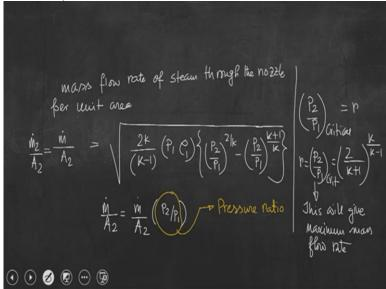
So the mass flow rate of steam through the nozzle per unit area  $=\frac{\dot{m}_2}{A_2}=\frac{\dot{m}}{A_2}$ So why I am writing  $\dot{m}$ ? Because from continuity we can write  $\dot{m}_1 = \dot{m}_2 = \dot{m}$ . So
