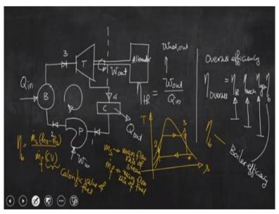
So this is the simplest schematic depiction of the steam power cycle or plant drawn in the slide. And we can see from this depiction that there are four major components; boiler, turbine, condenser and pump. So this B is used to denote boiler. We have discussed about the description of this particular diagram. We have also discussed about thermal efficiency of the cycle. That is nothing but
