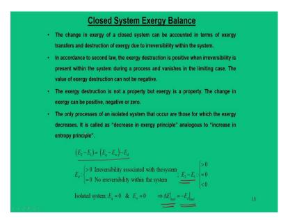
Now, here these equations has a very significant repercussions. First thing we are going to see here that this exergy change  $(E_2 - E_1) = (E_q - E_w) - E_d$ ,  $E_d$  is nothing but exergy destruction. So, this  $E_d$  can have 0 or it can be greater than 0. So, when it is 0 it means there is no irreversibility associated with the systems.
