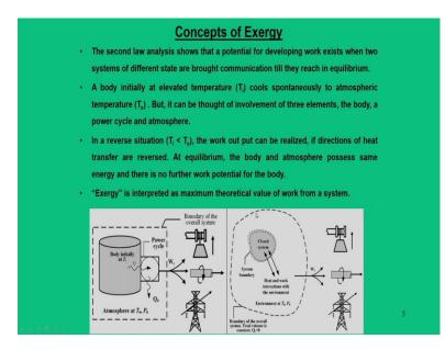
So, what we have seen here in this figure that we have a body which is initially at temperature  $T_i$  and we want to extract the work potential or we want to quantify its work potential. So, for that purpose it must reject heat to the atmospheres. So, the body which is at initial temperature  $T_i$  and whereas, we have this atmosphere and typically we call this as surroundings, it is maintained at temperature  $T_0$  and  $p_0$ .
