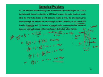
And the similar line we are now going to solve the second problem which is mainly on the exergy balance for the closed system. So, what the problem talks about is that in many industrial situations there is a heat generated in a furnace and we ensure that heat should not come out. So, that means, we provide sufficient insulation that heat should not come out and we have some arbitrary ambient conditions which is atmospheric conditions.
