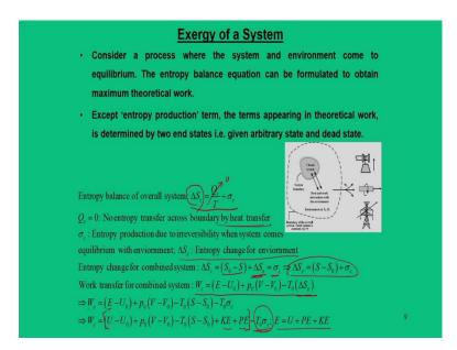
Now, for the same the situation what we did in the previous slide? It was the energy balance. Now we will be talking about the entropy balance. So, for the same figure we can write or recall the entropy balance of the overall system  $\Delta S_c = \frac{Q_c}{T} + \sigma_c$ . Now this  $\frac{Q_c}{T}$  is 0, because no entropy transfer across the boundary by heat transfer.
