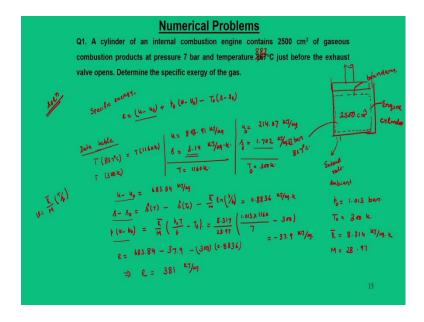
So, now we are at the end of this particular lecture we are now going to look into some numerical problems which will clarify some of our understanding and the first one which we are going to discuss is the exergy study for an IC engine. Normally when you say internal combustion engines we are very familiar that exhaust of an engine carries lot of energy.
